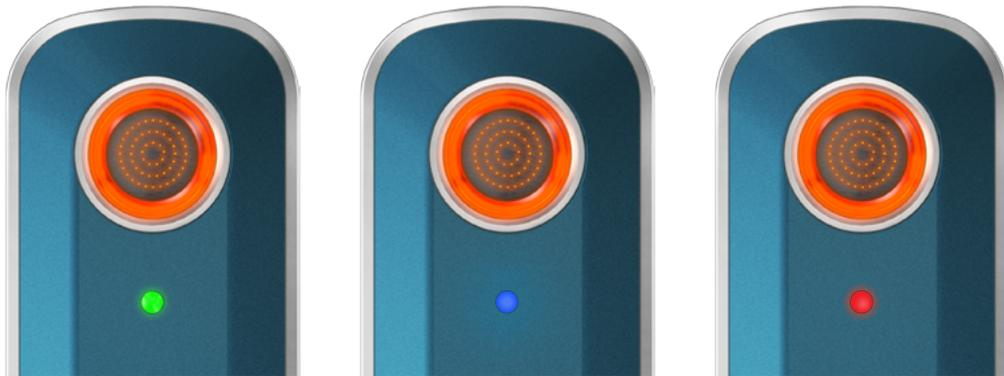
**Blinking Green:** Firefly2 is heating.
