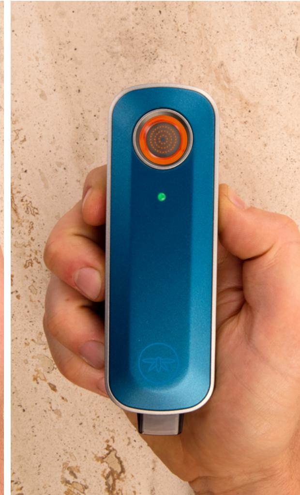
**PLEASE NOTE:** The Firefly will turn off after 30 seconds of holding the sensors, and the heating coil will not glow as bright towards the end of a vape session.
